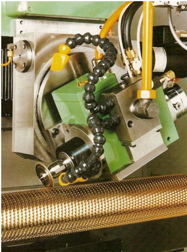
Fig.N°3- Resharpening of a broach of Sib Sideral- (Leini- Torino – Italy)
